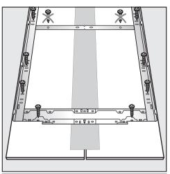
Please note: When attaching the mounting frame onto two adjacent doors (see "Front panel gap kit") screw into the thicker outer frames of the doors **only**.
